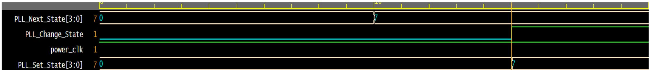
Case 1: VCD can be used to verify whether the Block is switching it's PowerState as expected and also the delay between transistions due to capacitance
