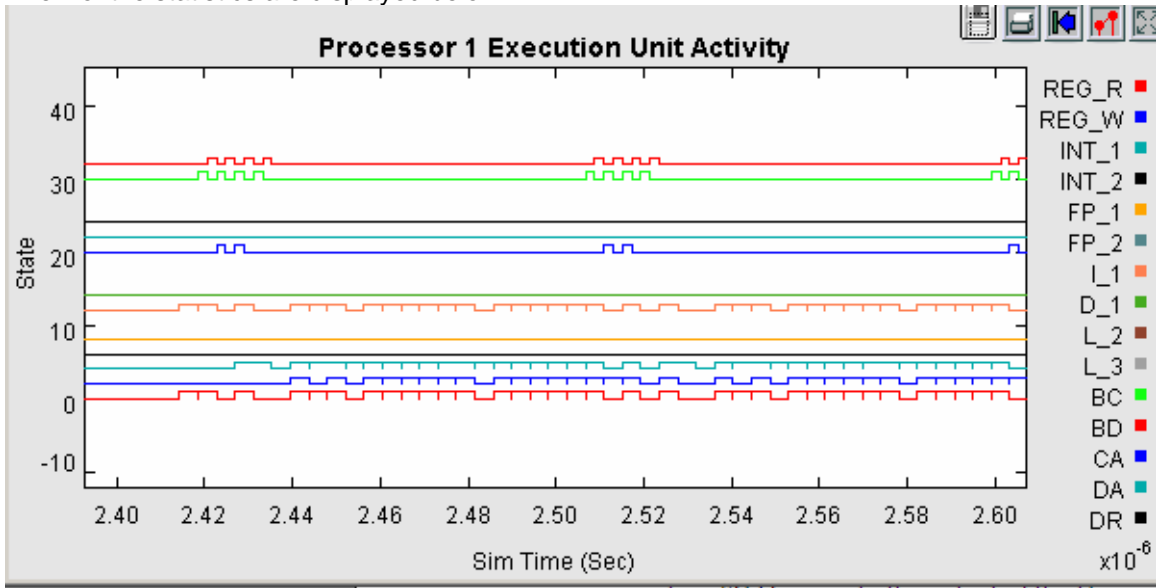
Figure 4 Timing Diagram of the SH4 Processor Resources
